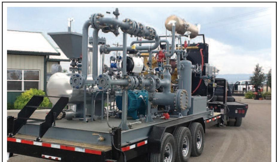
The multiphase blow down unit from Leistritz is a portable, self-contained system for removing liquids and gases from the wellbore while increasing well pressure. Connected to the well's export line, the unit draws down the well's back pressure to increase production stream velocity.
